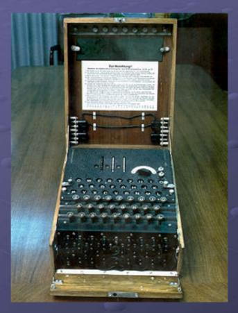
The plugboard, keyboard, lamps, and finger-wheels of the rotors emerging frm the inner lid of a three-rotor German military Enigma machine
